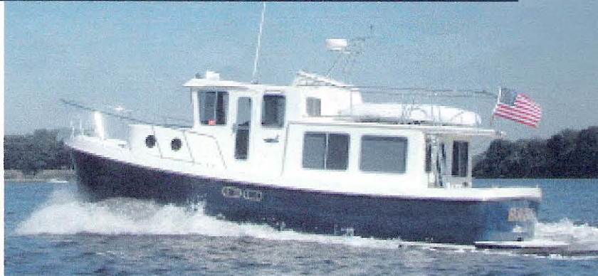
The American Tug 34 has a range of about 566 miles at its 12-knot cruising speed.
