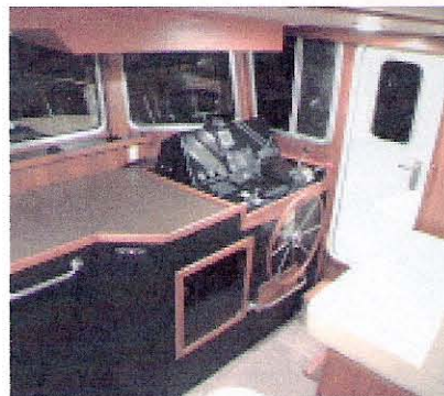
The pilothouse has its helm to starboard, with an expansive chart table and loads of room for electronics on the dash.
